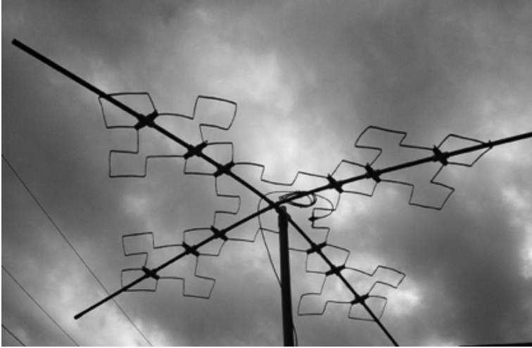
Figure 6. A fractal antenna.
